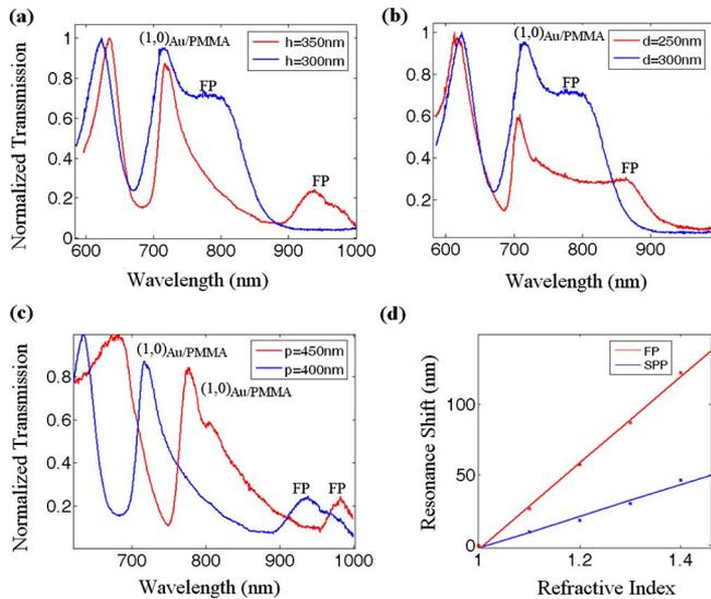
FIG. 4. (Color online) Comparison of spectrum (a) with changing dielectric layer thickness, (b) with changing diameter, and (c) with changing periodicity. (d) Shifts in spectral position with changing RI for FP peak (red) and  $(1,0)_{\text{Au/PMMA}}$  peak (blue).
