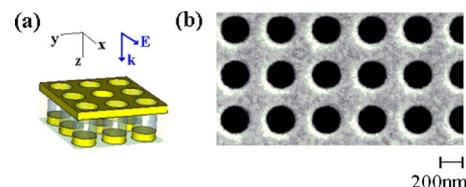
FIG. 1. (Color online) (a) Schematics of the multilayered plasmonic crystals; blue arrows show incident light configuration. (b) SEM image of a periodic array (diameter=250 nm and period=400 nm).
