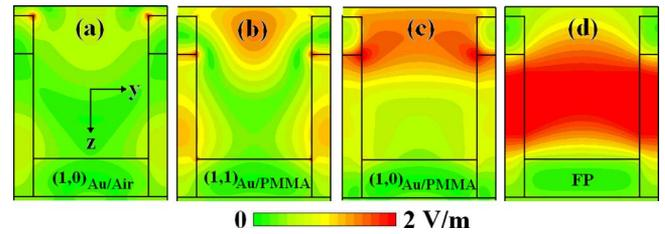
FIG. 3. (Color online) Cross sectional  $E_x$  field patterns are shown for (a)  $(1,0)_{\text{Au/air}}$ , (b)  $(1,1)_{\text{Au/PMMA}}$ , (c)  $(1,0)_{\text{Au/PMMA}}$ , and (d) FP peaks. Cross sections are obtained at resonance peaks ( $f_a = 575$  THz,  $f_b = 505$  THz,  $f_c = 434$  THz, and  $f_d = 320$  THz, respectively) using a Fourier transform. Simulation is done with a structure of 300 nm diameter and 400 nm periodicity.
