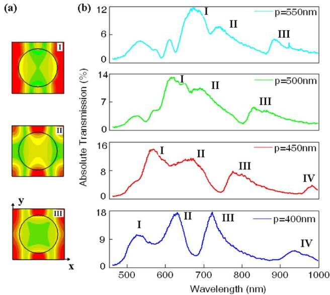
FIG. 2. (Color online) (a)  $H_y$  field patterns of  $(1,0)_{\text{Au/air}}$ ,  $(1,1)_{\text{Au/PMMA}}$ , and  $(1,0)_{\text{Au/PMMA}}$  are shown, respectively, from top to down. (b) The absolute transmission spectra of the structures for crystals with diameter ( $d = 300$  nm) and varying periodicities ( $p$ ) from 550 to 400 nm with 50 nm steps, respectively, from top to down.
