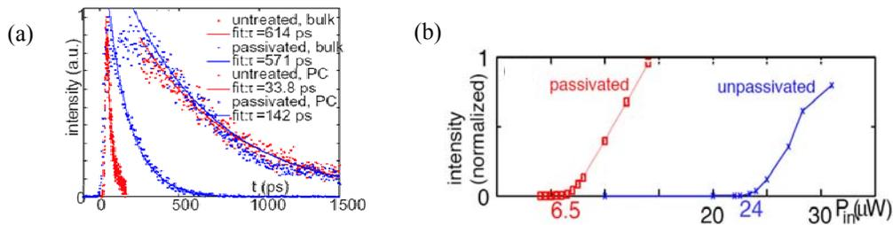
**Figure 1 (a-b)** PL measurements and lasing curve for the untreated (red) and passivated (blue) samples, from the PC and unpatterned regions at low temperature.
