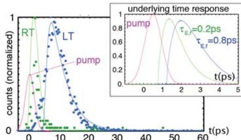
**Figure 2** Photonic crystal laser time response. (a) At low temperature (blue curve), FWHM=14.1 ps at  $2\times$  above lasing threshold. At room-temperature (green), time response follows that of the pump laser with FWHM=3.5 ps. Inset: Calculated response to a shorter, 1-ps excitation pulse shows FWHM near 1 ps when pumped  $2\times$  above threshold; response is faster if we assume faster carrier relaxation time  $\tau_{E,f}$ .
