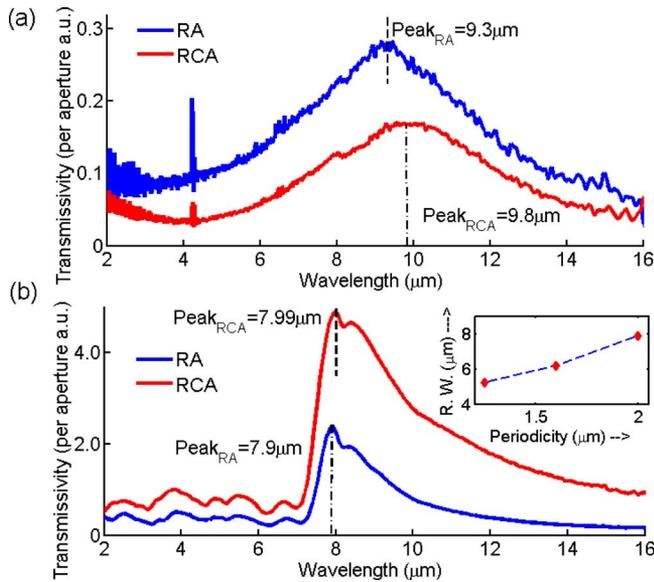
FIG. 2. (Color online) The transmissivity spectra for the (a) random and (b) periodic arrays of rectangular (blue) and RCA (red) nanoapertures are shown. Inset shows the periodicity dependence of the resonance peak for RA array.
