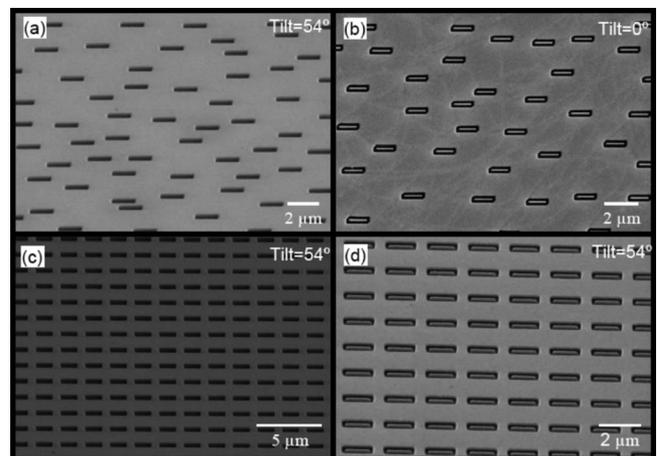
FIG. 1. Scanning electron images of random (a) rectangular and (b) RCA array are shown together with periodic arrays of (c) rectangular and (d) RCA arrays.
