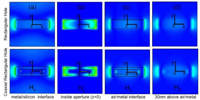
FIG. 3. (Color online) Dominant field profiles for the rectangular and RCA nanoapertures are shown (a) at metal/silicon interface, (b) in the middle of the nanoaperture, (c) at metal/air interface, and (d) 30 nm in air.
