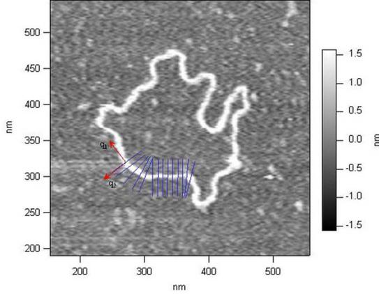
Fig. 1. AC-mode image of a DNA strand. Image courtesy of J. Park of the Rowland Institute at Harvard.
