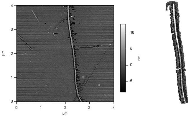
Fig. 2. Raster scan and local raster scan images of the same carbon nanotube. Note that most of the raster scan image is of the substrate while the local raster scan image is primarily of the nanotube. (Reprinted with permission from [36].)
