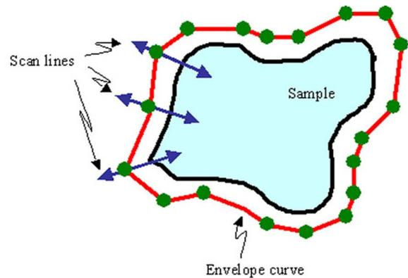
Fig. 5. An example of a sample and an envelope curve. The envelope curve is defined by a set of points. Associated to each point is a scan line. The AFM tip is moved along each scan line consecutively.
