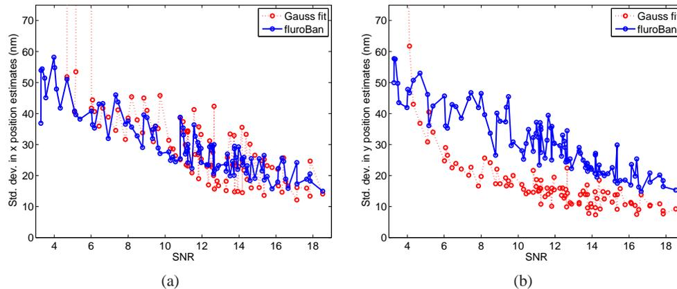
Fig. 5. Comparison of the standard deviation of the position estimate using fluoroBancroft (blue solid line) and Gaussian fit (red dashed line). (a) Standard deviation of the  $x$ -position estimate. (b) Standard deviation of the  $y$ -position estimate. In the  $x$ -direction, the two estimators are very similar while in the  $y$ -direction the Gaussian fit exhibits consistently better performance at SNRs above 6.
