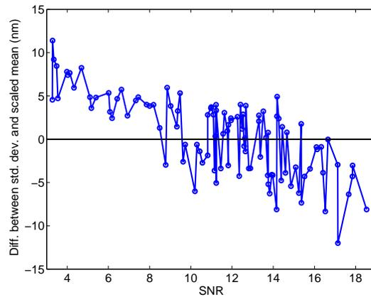
Fig. 4. Biasedness of the fluoroBancroft estimator. If the estimator were unbiased, then the mean and variance of the displacement estimates would be related by (21). That the difference, shown here, is not zero indicates the algorithm exhibits some bias in the position estimates.
