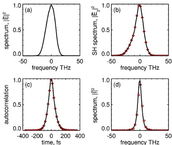
FIG. 2. (Color online) Measured experimental data (solid lines) used for retrieval of the pulse shape. Symbols are calculated using the retrieved electric field. (a) Fundamental spectral intensity, (b) second harmonic spectral intensity, (c) intensity autocorrelation, and (d) Fourier transform of intensity autocorrelation.
