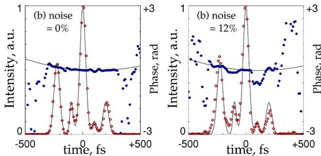
FIG. 4. (Color online) Reconstruction simulations of a complicated pulse in the presence of (a) no noise, and (b) intensity noise=12%. Solid lines correspond to original pulse and symbols (diamonds are intensity, and filled circles are phase) represent reconstruction results.
