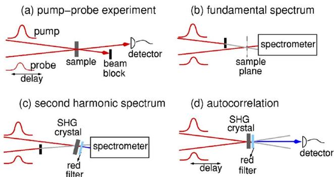
FIG. 1. (Color online) Schematic of a pulse characterization scheme at the sample site in a pump-probe experiment. (a) Typical pump-probe setup, (b) measurement of fundamental spectrum, (c) second harmonic spectral measurement, and (d) intensity autocorrelation.
