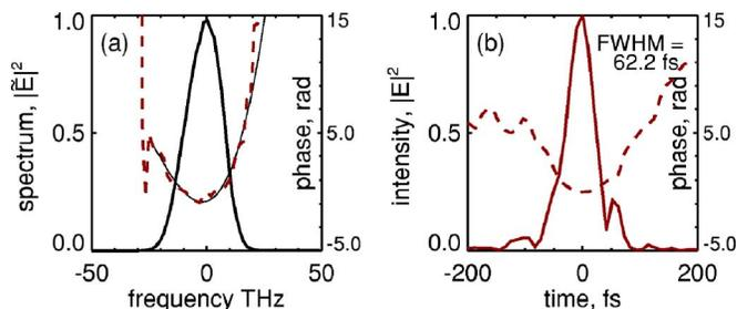
FIG. 3. (Color online) Reconstruction results. (a) Measured spectral intensity (thick solid line) and adapted phase (dotted line). (b) Temporal intensity and phase of the retrieved optical pulse.
