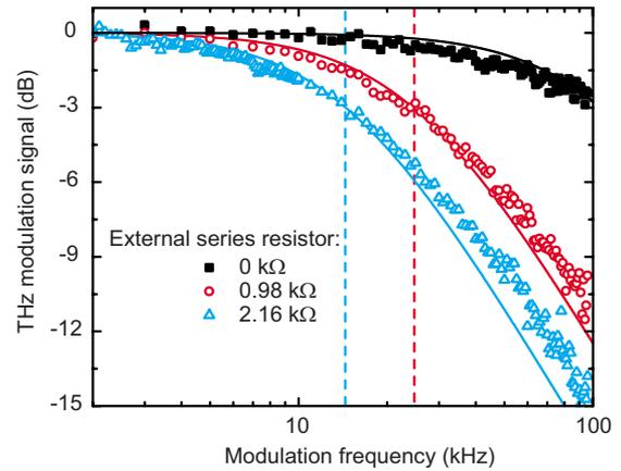
FIG. 3. (Color online) Terahertz modulation signals of device A as a function of the modulation frequency when loaded with various external series resistors. The solid curves are  $RC$  fits to the experimental data.
