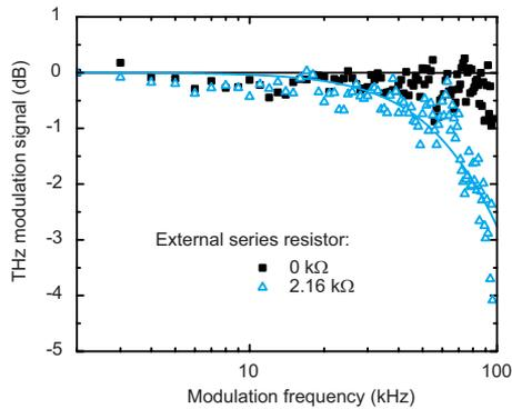
FIG. 4. (Color online) Terahertz modulation signals of device B as a function of the modulation frequency when loaded with 0 and 2.16 k $\Omega$  external series resistors. The solid curves are fits to the experimental data.
