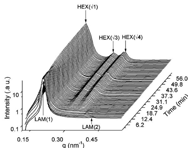
**Figure 3.** The time-evolution of SAXS intensity following a  $T$ -jump from 155 to 120 °C. The triblock copolymer SEBS transformed from LAM phase into HEX phase within 20 min.
