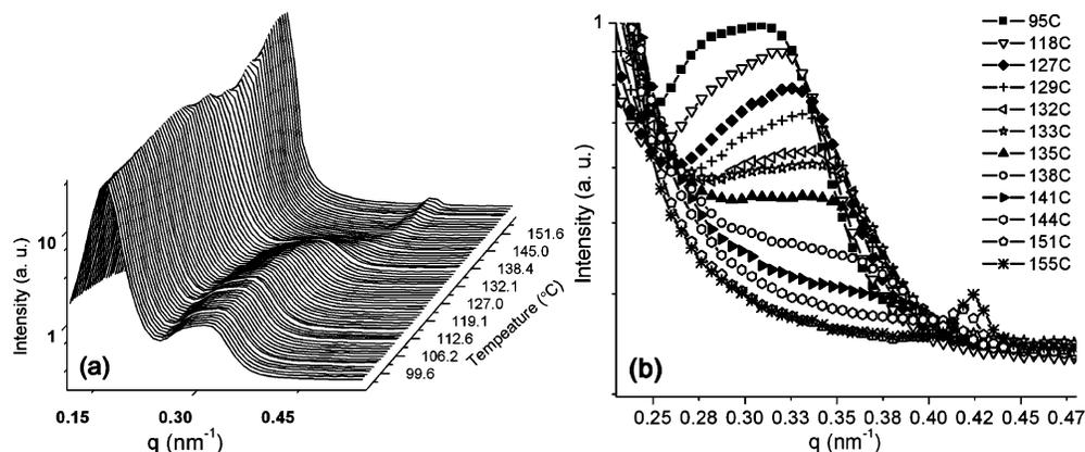
**Figure 2.** (a) Time-resolved SAXS data collected during a temperature ramp from 95 to 155 °C at a rate of 1 °C/min. (b) Several frames in the  $q$  range of 0.23–0.48 nm<sup>-1</sup> at different temperatures are selected from the data shown in panel a to identify the transition temperature. The OOT temperature was located around 135 °C according to this temperature ramp experiment.
