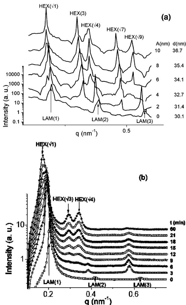
**Figure 10.** (a) The scattering intensity calculated from the model using 200 lamellae of thickness  $L = 20$  nm with wavelength  $\lambda = 42$  nm. The length of the lamellae along the direction of the wave was set to  $50\lambda$ . The fluctuation amplitude  $A$  was varied from 0 to 10 nm and the spacing  $d$  from 30.1 to 36.7 nm as indicated. (b) Time-resolved SAXS data of Figure 4a are reproduced here for comparison.
