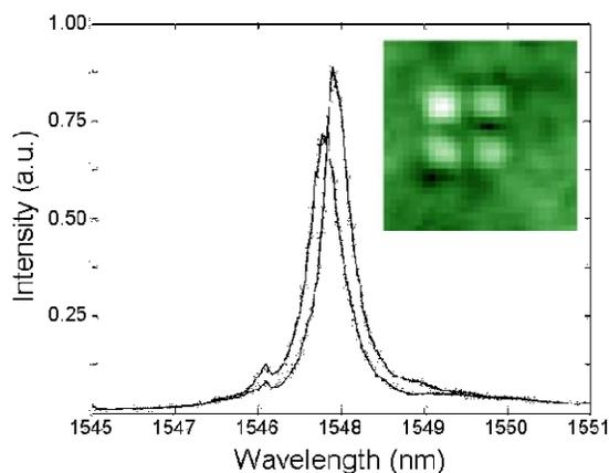
**Fig. 2: Recorded resonant curves for two pixels. Shift indicates a 5-nm difference in height. (Insert) A 2-D image where brightness indicates the surface height at every location. Four box features can be seen. Measured boxes deviate from actual dimensions by 0.7 nm RMS.**
