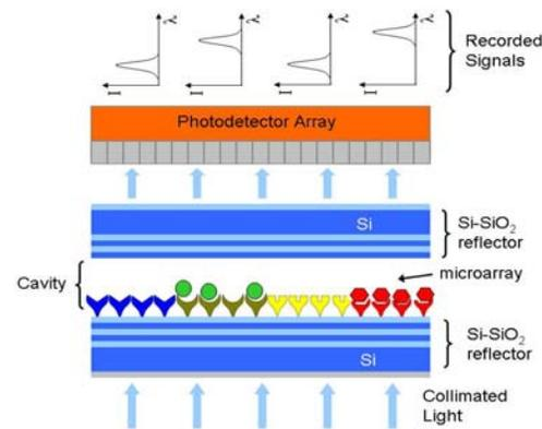
**Fig. 1** The wavelength of the excitation light swept and wavelength vs. transmission curves are recorded by a camera positioned beyond the cavity. The microarray is fabricated on one of the reflector surfaces. Binding to the surface is indicated by a local shift in the resonant response of the cavity.
