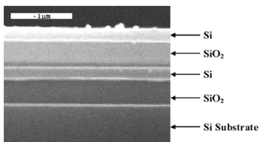
**Fig. 3: Cross-sectional SEM of reflecting (double SOI) substrate**
