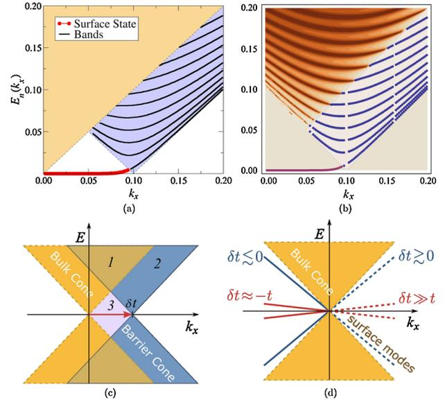
FIG. 3 (color online). (a) Dispersion of the confined solutions  $E_n(k_x)$  for  $\delta t = 0.1$  and  $L = 200$ . (b) A density plot of the transmission  $t(E, k_x)$  from Eq. (5) is shown in the upper region (region 1), which is plotted together with the same data as in panel (a). (c) Regions 1, 2, and 3 discussed in the text. (d) Linearly dispersing modes for the narrow barrier discussed in the text.
