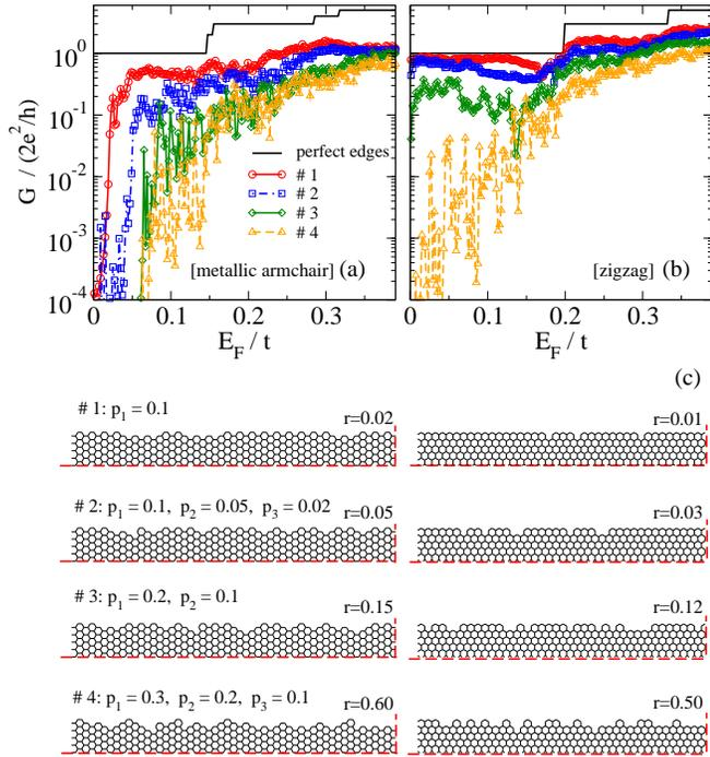
FIG. 2: (Color online) (a) and (b): Energy dependence of the average linear conductance of graphene nanoribbons with varying edge roughness. All nanoribbons have a the same length ( $L = 45$  nm) and similar widths ( $W = 4.4$  nm for armchair and  $W = 4.7$  nm for zigzag). (c) Typical etching profiles used in (a) and (b) (only segments of the nanoribbon atomic structure are shown). Left: armchair and right: zigzag.
