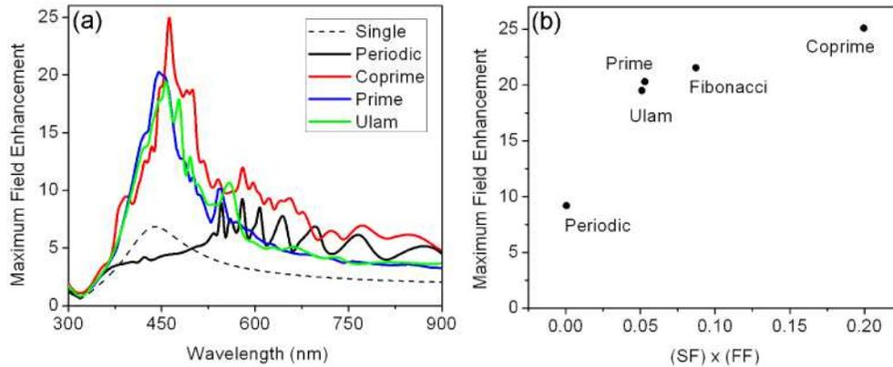
Fig. 3. (a) Maximum field enhancement versus the wavelength for an isolated particle, and for Periodic, Coprime, Prime, and Ulam arrays. The arrays are excited by a circularly polarized plane wave at normal incidence. (b) Values of maximum field enhancement versus the spectral flatness (SF) – filling fraction (FF) product for the different arrays indicated in the figure.
