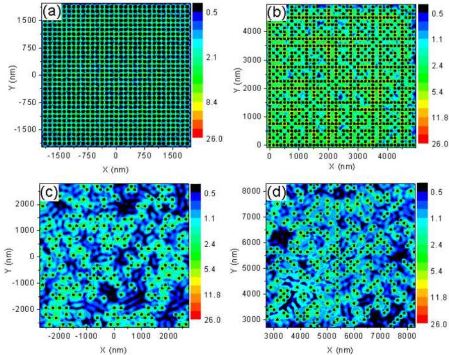
Fig. 4. Field enhancement spatial distribution (logarithmic scale) on the array's plane at the frequencies of the maximum field enhancement: (a) periodic at 580nm (b) Coprime at 462nm (c) Prime at 439 nm (d) Ulam at 450 nm. The arrays are excited by a circularly polarized plane wave at normal incidence.
