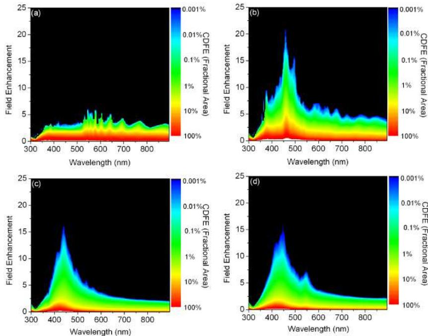
Fig. 5. The color-maps show the cumulative distributions of field enhancement (CDFE) (logarithmic scale) versus wavelength (x-axis) and field-enhancement (y-axis) for (a) Periodic (b) Coprime (c) Prime and (d) Ulam arrays. The arrays are excited by a circularly polarized plane wave at normal incidence.
