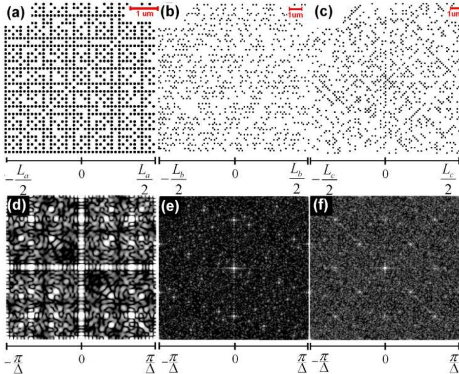
Fig. 2. Aperiodic arrays (a-c) and their corresponding structures in the reciprocal space (logarithmic scale) (d-f): (a) and (d) Coprime  $L_a=4.9\mu\text{m}$ , (b) and (e) Prime  $L_b=10.5\mu\text{m}$ , (c) and (f) Ulam  $L_c=11\mu\text{m}$ . The dimensions of the reciprocal space are the same as in the periodic case (Fig. 1(b)) since the minimum center to center inter-particle distance ( $\Delta$ ) is equal to the periodic case.
