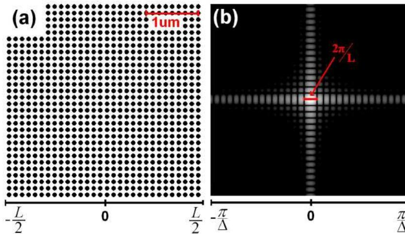
Fig. 1. Periodic array and its structure in the reciprocal space (logarithmic scale), where  $L = 3.75$  and  $\Delta$  is the center to center inter-particle distance, namely  $\Delta = d_{\text{min}} + 2r$ . The reciprocal space is obtained by the discrete Fourier transform (DFT). The width of the central peak in the reciprocal space is inversely proportional to the array's dimension.
