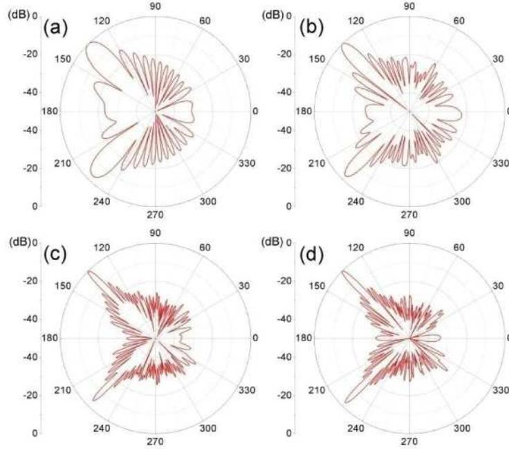
Fig. 10. Magnitude, in the Fraunhofer zone, of the scattered E-field in a plane orthogonal to the array and including the lattice's vertical axis, for different geometries, excited by a plane wave, propagating at the wavelength of the scattering efficiency's maximum: (a) Periodic at 580nm (b) Coprime at 462nm (c) Prime at 439 nm (d) Ulam at 450 nm. The incoming plane wave is at 45° incidence and is circularly polarized. The plots are in dB scale.
