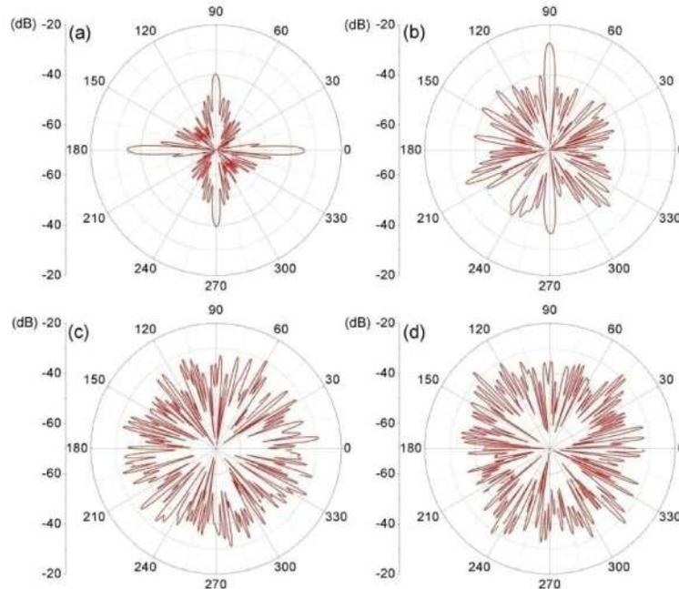
Fig. 11. Magnitude, in the Fraunhofer zone, of the scattered E-field in the array's plane, for different lattices excited by a plane wave at the frequencies of the scattering efficiency's maxima: (a) Periodic at 389.5nm, (b) Coprime at 462nm, (c) Prime at 439nm (d), and Ulam at 450.5nm. The incoming plane wave has a wave vector orthogonal to the array's plane and is circularly polarized. The plots are in dB scale.
