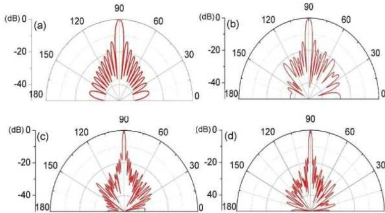
Fig. 9. Magnitude, in the Fraunhofer zone, of the scattered E-field in a plane orthogonal to the array and including the lattice's vertical axis, for different geometries, excited by a plane wave, propagating at the wavelength of the scattering efficiency's maximum: (a) Periodic at 580nm (b) Coprime at 462nm (c) Prime at 439 nm (d) Ulam at 450 nm. The incoming plane wave is at normal incidence and is circularly polarized. The plots are in dB scale.
