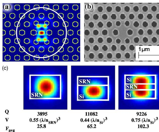
FIG. 1. (Color online) (a) Electric field magnitude of the  $x$ -dipole mode of a modified S1 defect cavity in the center of the slab and (c) in cross section for SRN, Si/SRN, and Si/SRN/Si membrane designs. (b) Scanning electron microscope image of the fabricated photonic crystal cavity.
