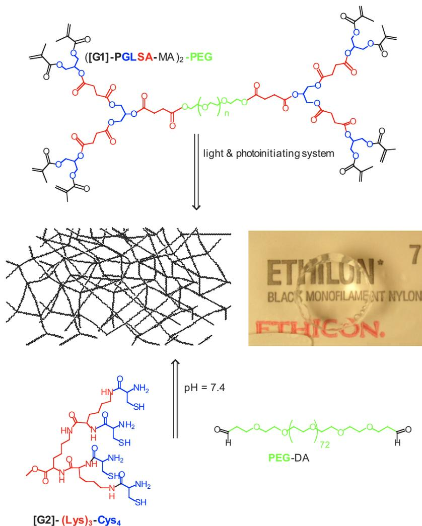
Fig. 4. Schematic of the two crosslinking strategies: (top) photocrosslinking reaction and (bottom) nucleophile–electrophile reaction.
