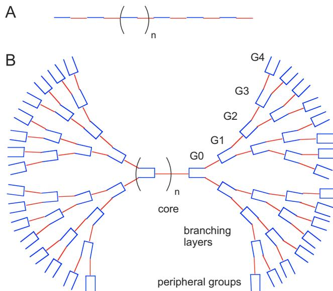
Fig. 1. Schematic of a linear (A) and dendrimer (B) polymer. The three main structural zones of the dendrimer consisting of the central core, internal branching layers, and peripheral groups are labeled.
