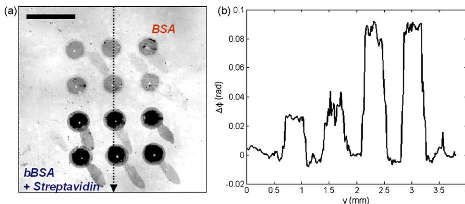
**Fig. 3.** SD-OCPM protein assay on selective absorption of streptavidin to bBSA. The BSA and bBSA were spotted on the sensor surface. After incubation with streptavidin solution and rinsing with PBST, a  $\sim 0.055$  rad increase in phase delay was observed on bBSA spots, relative to BSA spots. (a) SD-OCPM image on sensor chip. The scale bar represents 1 mm. (b) Phase distribution along the line indicated in (a).
