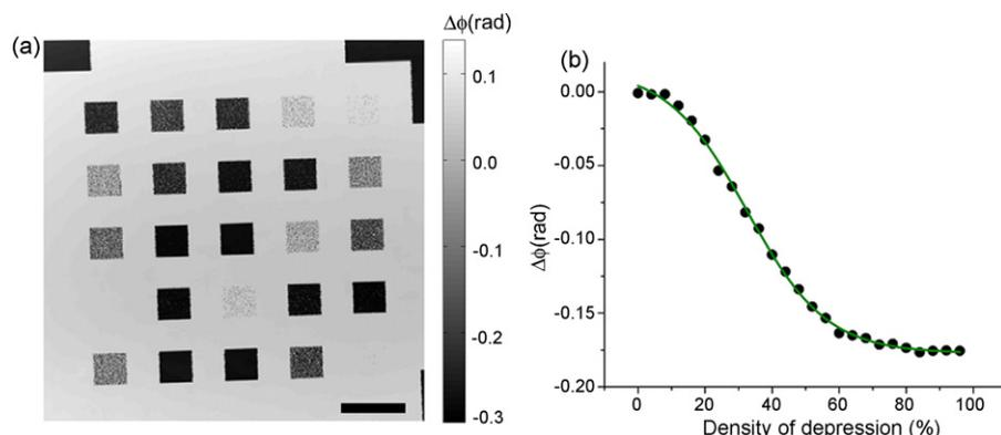
Fig. 2. (a) SD-OCPM phase image of 5 × 5 SiO<sub>2</sub> square etch patterns. Each square has a size of 100 μm × 100 μm. The maximum etch depth was ~7 nm. The scale bar denotes 200 μm. (b) Etch depth vs. depression level (0% depression level corresponds to no etching in the region).
