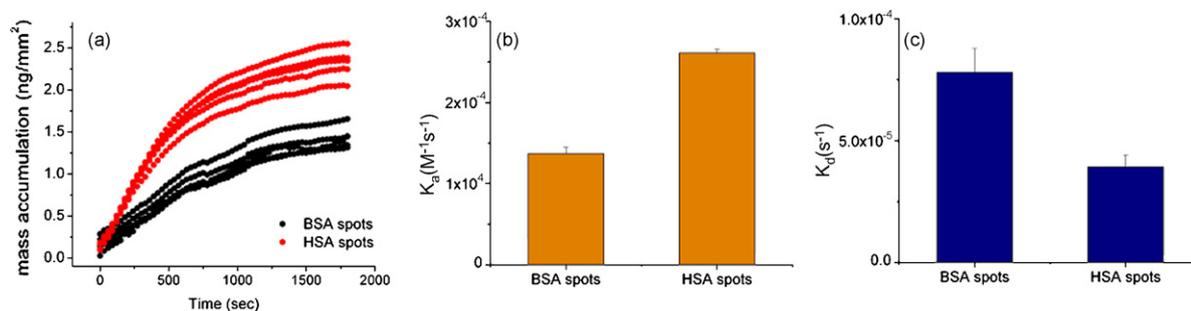
**Fig. 5.** Calculated kinetic association and dissociation parameters for BSA and HSA spots with  $\alpha$ HSA. (a) Sensorgrams for each spot and (b and c) present  $k_a$  and  $k_d$  averaged over 5 spots for each species. The error bar denotes standard deviation.
