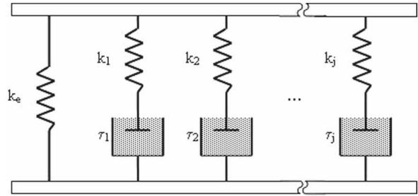
FIG. 1. Maxwell–Wiechert spring-dashpot model.
