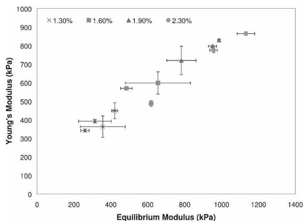
FIG. 7. The average Young's and equilibrium modulus at each nanoindentation position is shown above. Each point on the graph represents a single position on a gel and each gel is shown with a different data marker. Error bars are shown for both the Young's modulus and equilibrium modulus at each position. Two to five indents were performed at each position.
