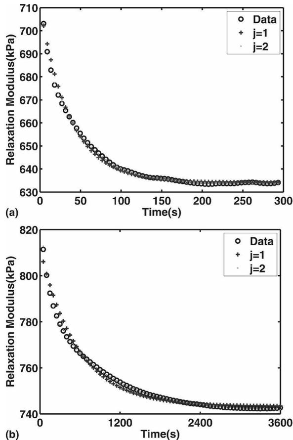
FIG. 8. Typical curve fits for Maxwell–Wiechert Model. (a) On nanoindentation data. (b) On unconfined compression data. For  $j = 1$ , the Maxwell–Wiechert model is equivalent to the standard linear solid (SLS) model. Both tests were performed on the same 1.6% pHEMA gel. Only every 100th data point is plotted for readability.
