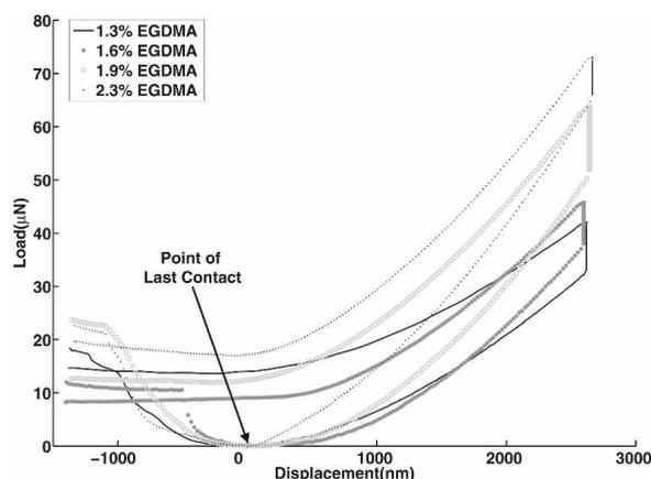
FIG. 3. Examples of load–displacement data for each of the four cross-linker concentrations. As expected, we see an increase in load with increasing cross-linker concentration for four indents with the same displacement. With these hydrated pHEMA samples, we do not see the snap-to-contact feature often seen with adhesive materials. As a result, the curves were offset so the point of last contact (minimum load on the unloading curve) was set to zero displacement and zero load.
