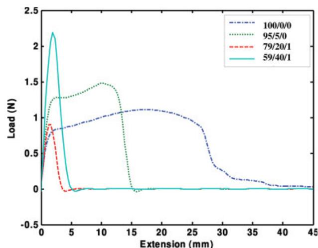
**Figure 6.** Average force-displacement curves ( $n = 10$ ) for each of the pressure sensitive adhesives tested. Error bars are omitted for clarity. [Color figure can be viewed in the online issue, which is available at [www.interscience.wiley.com](http://www.interscience.wiley.com).]
