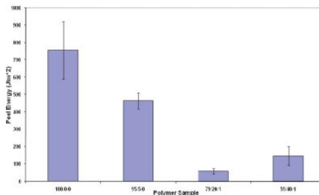
**Figure 5.** Work of adhesion, or peel energy, for each of the pressure sensitive adhesives. [Color figure can be viewed in the online issue, which is available at [www.interscience.wiley.com](http://www.interscience.wiley.com).]
