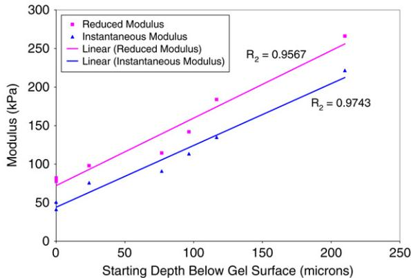
**Fig. 3 – The effect of starting depth on the calculated modulus of PuraMatrix-Collagen gels. The reduced modulus was calculated from an Oliver-Pharr fit to the unloading curve. The instantaneous modulus was calculated from a Maxwell-Wiechert fit to the stress relaxation curve.**
