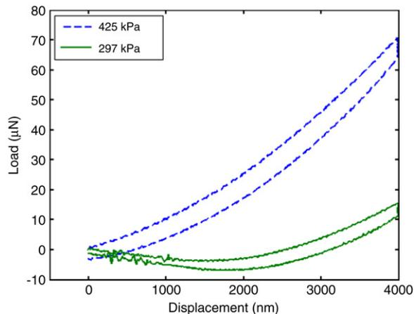
**Fig. 2** – Two examples of indents at the same position in the same PHEMA hydrogel. The first indent (dashed blue line) began with the tip below the sample surface. The second indent (green solid line) began in the water above the sample. Note the large error (43%) in the reduced modulus values from the Oliver–Pharr curve fitting method.
