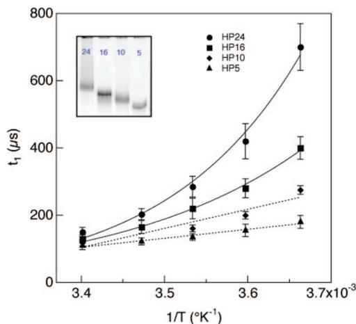
**Figure 4.** Unzipping times extracted from the dwell-time distributions, as a function of temperature for duplexes in the range 5–24 bp. Solid lines represent Arrhenius fits and dashed lines are linear approximations to the data. The inset displays a PAGE of the four hairpin molecules, stained using dsDNA stain SYBR Green I.
