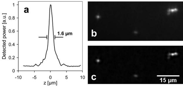
Fig. 3. a, Integrated signal from a thin fluorescent plane as a function of defocus  $z$ . b, Uniform-illumination image of  $1 \mu\text{m}$  beads (Molecular Probes TetraSpeck Slide B). c, Processed hybrid image from speckle and uniform illumination.
