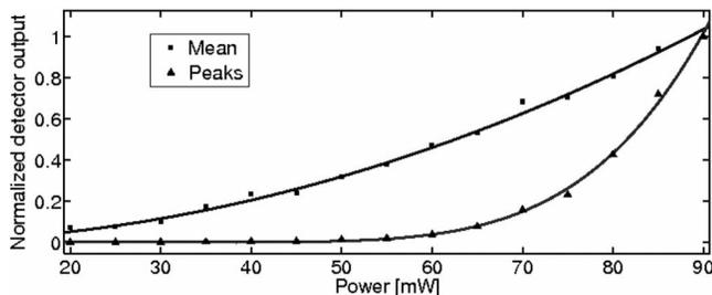
Fig. 1. A laser beam (1064 nm) is focused onto a bialkali PMT photocathode to generate thermionic emission. Peak counts (triangles) or the mean of the output (squares) are plotted against laser power. Solid curves indicate fits to the Richardson equation and to a quadratic, respectively.
