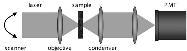
Fig. 2. TD-ACM schematic. A focused laser beam is scanned across a sample. Light transmitted through the sample is collected and focused onto the photocathode of a PMT. The resulting thermionic current is amplified by the PMT and then fed into a peak counting circuit to obtain  $J$ , or integrated to obtain the mean.
