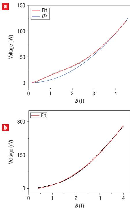
**Figure 3** The response of devices with and without the FM–NM interface.
