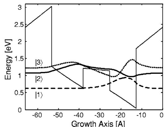
FIG. 1. Calculated conduction-band lineup and envelope functions of the three lowest bound states (referenced to their respective energy levels) of an AlN/GaN/AlGaN CQW structure, corresponding to sample A of Table I.
