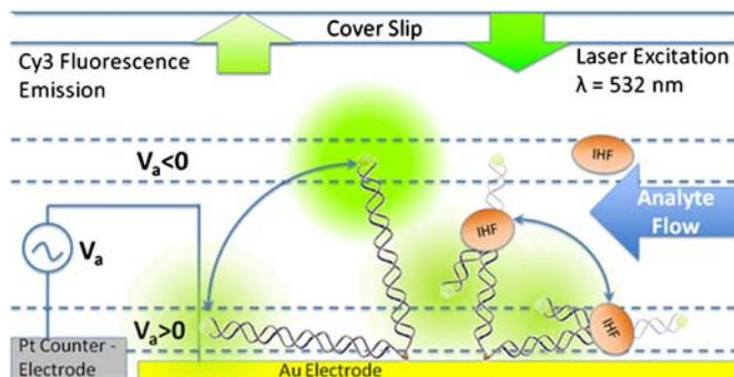
**Fig. 1.** Application of a negative potential repels the DNA probe from the surface and results in high fluorescence intensity because of inefficient ET between Cy3 and the gold electrode, whereas positive potentials pull the DNA probes to the surface, resulting in reduced fluorescent intensity.
