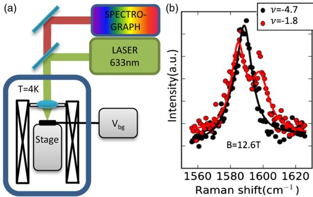
FIG. 1 (color online). (a) Schematic view of the cryogenic Raman setup using linearly polarized light. (b) *G*-band Raman spectra at  $B = 12.6$  T. Black spectrum measured at  $\nu = -4.7$  ( $V_{\text{bg}} = -20$  V). The red spectrum shows visible splitting of the *G* band at  $\nu = -1.8$  ( $V_{\text{bg}} = -8$  V). Solid lines are double-peaked Lorentzian fits.
