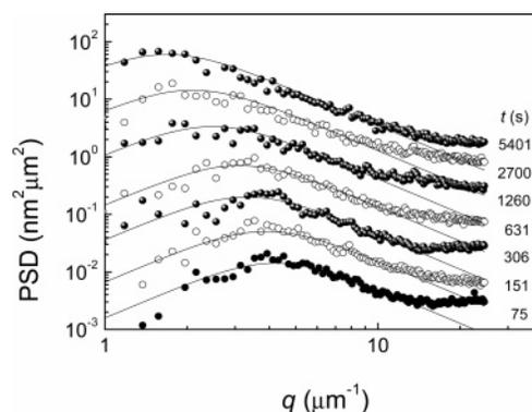
**Figure 2.** A subset of time-sequenced PSD, after background subtraction by  $A_q^2(0)\Theta(q^* - q)$  with  $q^*$  being  $3 \mu\text{m}^{-1}$ , of a 18 nm thick 2.3 kg/mol PS film obtained at different times upon annealing at 373 K. The solid lines are obtained by fitting the range of the PSD raw data that have grown above  $A_q^2(0)$  to eq 4 as described in the text.
