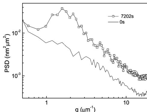
**Figure 1.** Power spectral density of an  $h_0 = 18$  nm and  $M_w = 2.3$  kg/mol spin-cast PS film, freshly prepared and after annealing for 7202 s.
