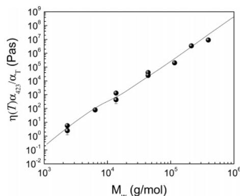
**Figure 4.** Measured values of  $\eta(T)$  divided by the corresponding shift factor,  $a_T$ , given in Table 1, plotted as a function of the molecular weight of the polymer films ( $\bullet$ ). The data of the highest molecular weight film ( $M_w = 940$  kg/mol) is not shown because the measurement time was not long enough to realize the  $\mu_0 \sim 1/t$  behavior (Figure 2b). The solid line represents the published data of the viscosity of bulk PS at 423 K.<sup>24</sup>
