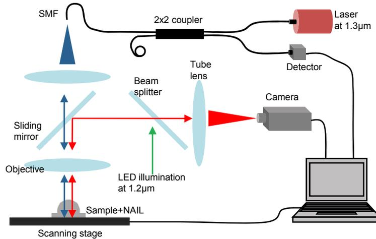
Fig. 1. (Color online) Experimental setup. A sliding mirror provides switching between confocal and widefield microscopes. When the sliding mirror is out, in confocal imaging, illumination and detection is done through the same fiber using a 2x2 optical coupler. When the sliding mirror is in, the sample is illuminated with an LED array and the image is captured using an InGaAs camera.
