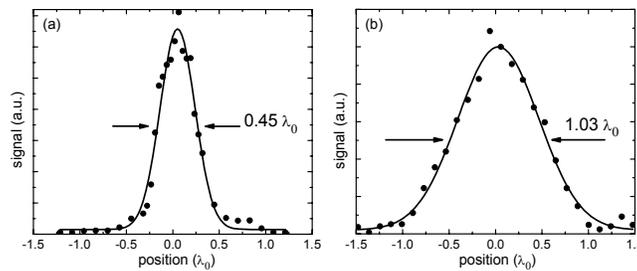
Fig. 5. Longitudinal linecut taken (a) with the confocal microscope and (b) with the wide-field microscope.
