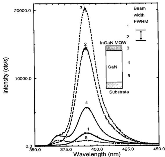
FIG. 3. Photoluminescence spectra ( $PL_{\text{edge}}$ ) of InGaN/GaN multiple quantum well structure as a function of position across the layer structure. The numbers in the inset figure represent the position of the corresponding spectra.
