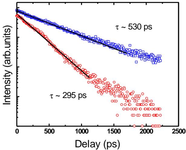
FIG.2. Time-resolved photoluminescence spectra at 4 K (log-linear scale). The square represents the data for free excitons and the circle represents the donor bound exciton. The solid lines are single exponential fits to the data.
