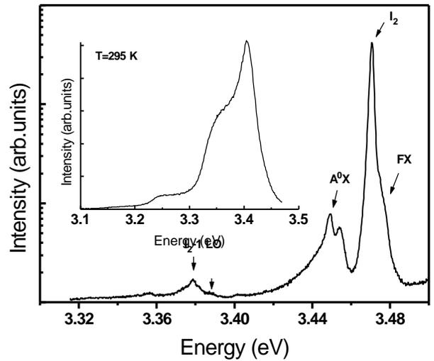
FIG.1. Time-integrated photoluminescence at 4 K (log-linear scale) and room temperature (linear-linear scale).
