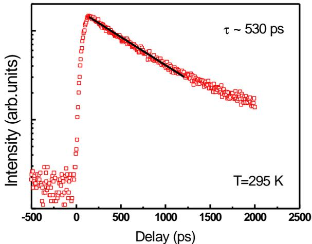
FIG.3. Time-resolved results for free excitons at room temperature (log-linear scale). The solid line is a single exponential fit to the data.
