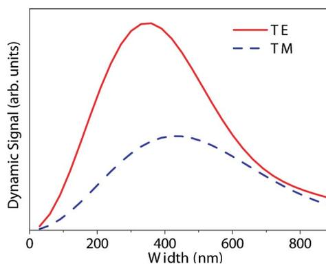
Fig. 3. (Color online) Normalized dynamic signal in the scattered field due to a focus superposition of evanescent waves with a FWHM spot size of 250 nm centered on the strip, at height  $\Delta=100$  nm, due to an oscillation of amplitude  $\delta\Delta=0.5$  nm, for both TE and TM polarization of the incident field.
