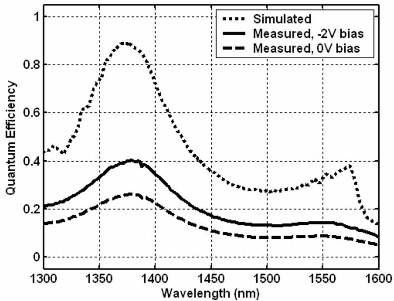
Figure 6: Measured Ge/DSOI photodetector QE at 0V and 2V reverse bias vs. simulated QE. The 140 μm by 140 μm area device includes a 737 nm Ge layer, capped with a 300 nm SiO<sub>2</sub> layer. Simulation assumes 100% carrier collection.
