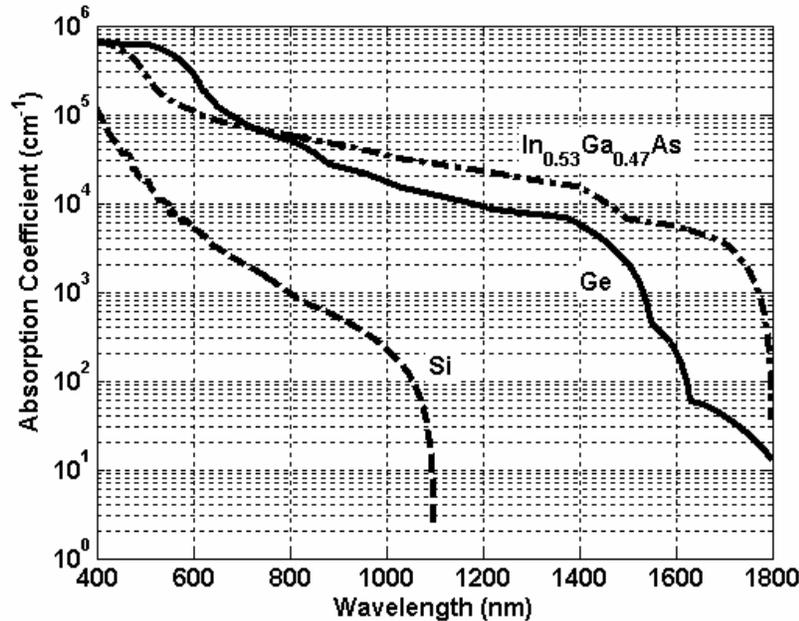
Figure 1: Absorption coefficients for various semiconductors
