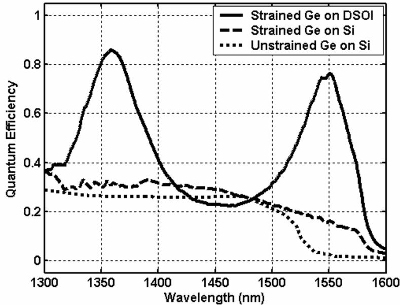
Figure 4: QE simulation of the Ge/DSOI photodetector optimized for 1550 nm operation, compared to both strained and unstrained Ge/Si; Ge thickness: 860 nm. Simulations assume 100% carrier collection.
