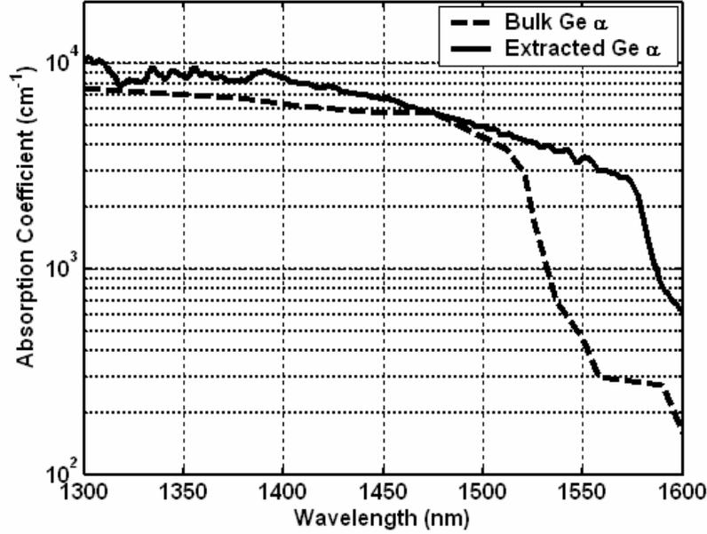
Figure 3: A comparison of the extracted strained-Ge absorption coefficients to bulk-Ge values. Extracted values were from an undoped Ge/Si sample, and bulk-Ge values were obtained from Ref. 12.
