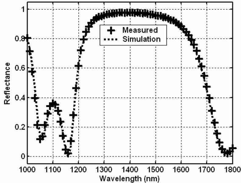
Figure 2: Simulated and measured reflectivity of the DSOI structure in the NIR
