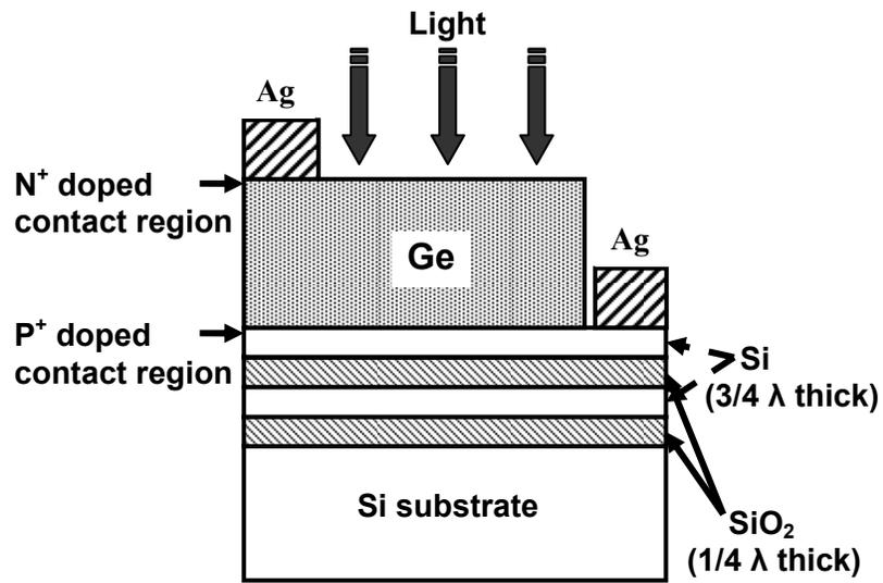
Figure 5: Cross-sectional view of the top-illuminated Ge/DSOI vertical PIN photodetector; Ge thickness: 755 nm.
