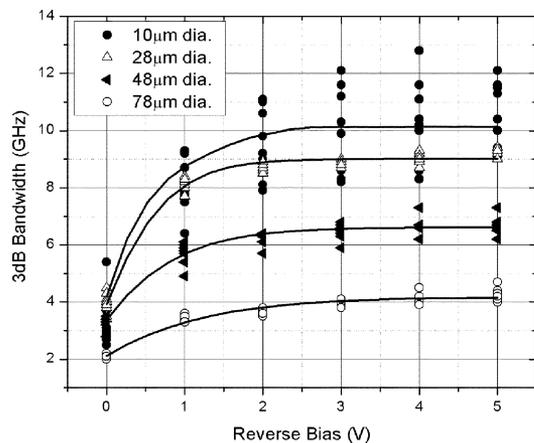
Fig. 4. 3-dB bandwidth at 1550 nm versus reverse bias for Ge-SOI detectors of sizes 10, 28, 48, and 78  $\mu\text{m}$  in diameter. Empirical fit curves for each detector size group are included as trend lines.
