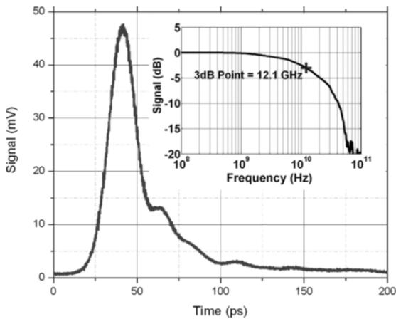
Fig. 3. Temporal response of a 10- $\mu\text{m}$  diameter detector at  $-3\text{-V}$  bias and 1550-nm wavelength. Measured pulse FWHM is 20 ps. FFT of the temporal response is illustrated in the inset, which shows the 3-dB point at 12.1 GHz.
