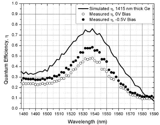
Fig. 2. Simulated versus measured  $\eta$  of a 78- $\mu\text{m}$  diameter Ge-SOI photodetector, resonant at 1538 nm. The measured  $\eta$  at 0- (open circles) and -0.5-V bias (filled circles) are illustrated.
