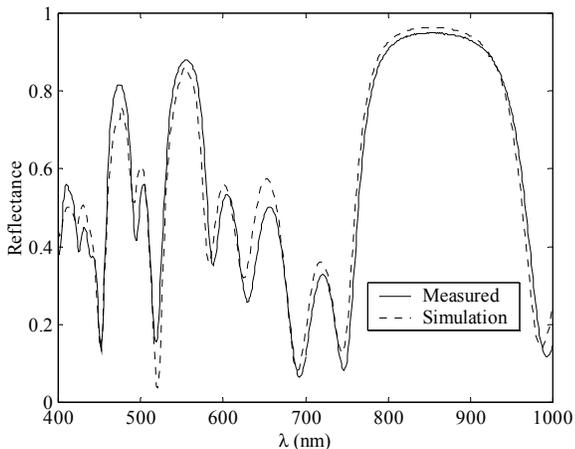
Fig. 2. Reflectivity of two period distributed bragg reflector showing excellent fit with simulated results.
