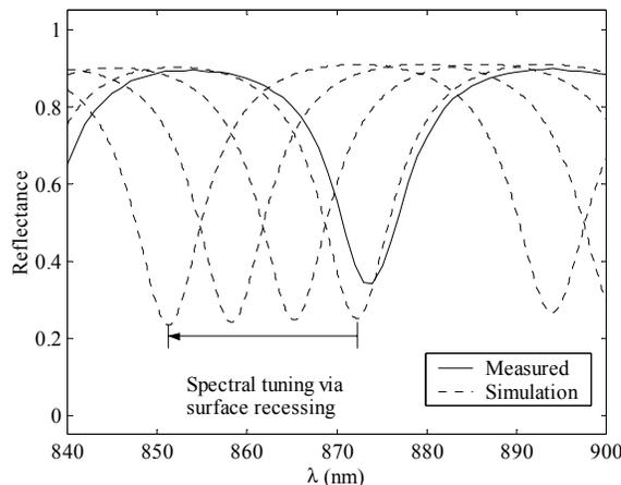
Fig. 4. Simulated effect of surface recessing for use in spectral tuning of the reflectance minima.
