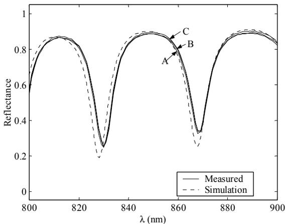
Fig. 3. Reflectivity of final silicon wafer (acquired at three random locations on wafer) with buried distributed Bragg reflector.
