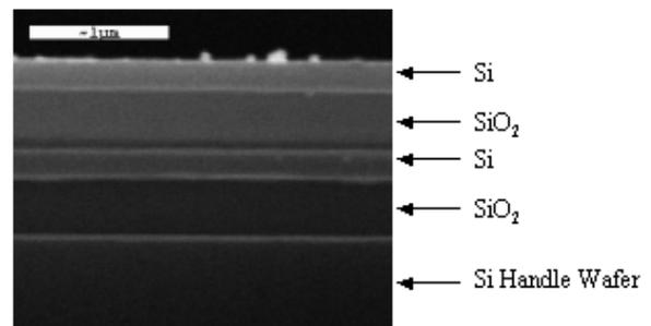
Fig. 1. Cross-sectional SEM of reflecting silicon substrate showing buried distributed Bragg reflector.
