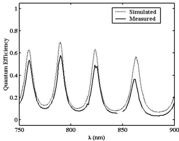
Fig. 2. Spectral quantum efficiency of RCE pin photodetector.
