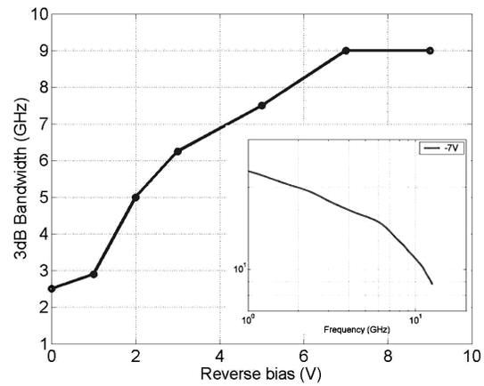
Fig. 4. Frequency bandwidth of 30- $\mu\text{m}$ -diameter device at various bias values calculated from temporal response. The inset shows the bode plot for 7 V reverse bias.
