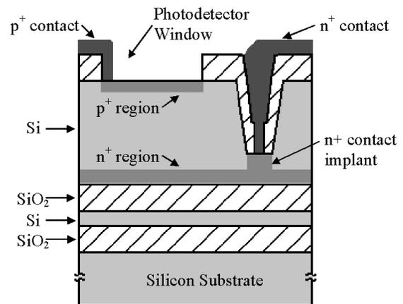
Fig. 1. Cross-section of RCE Si pin photodetector showing trench via for buried n+ contact.
