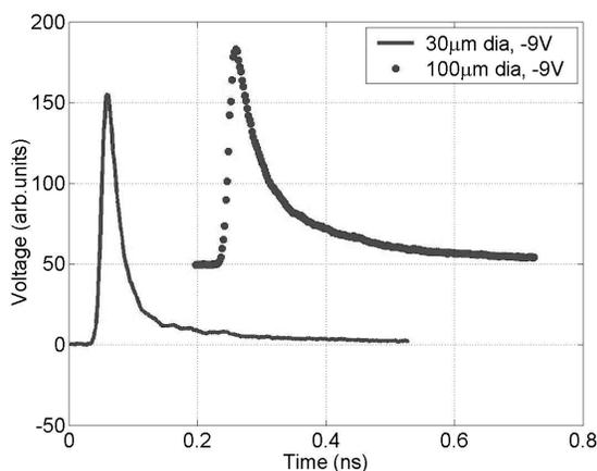
Fig. 3. Measured temporal responses of 30  $\mu\text{m}$ - and 100  $\mu\text{m}$ -diameter photodiodes.
