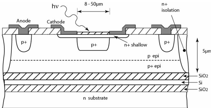
Fig. 1 Cross section of the RCE-SPAD structure.
