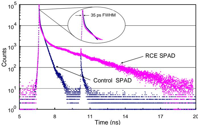
Fig. 3 Time response of RCE and control SPAD detectors to a picosecond laser pulse at 820nm (the small secondary peak occurring at  $\sim 10\text{ns}$  is due to a reflection at the fiber connector). Both SPADs have an active area diameter of  $50\mu\text{m}$  and are operated at 5V excess bias voltage.
