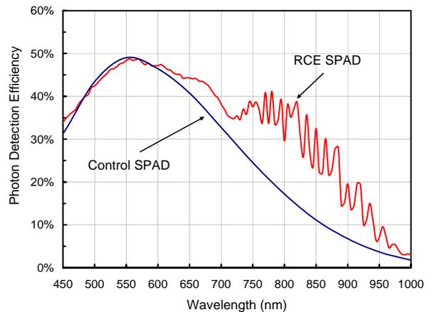
Fig. 2 Photon detection efficiency of RCE and control SPAD detectors at 5V excess bias voltage.
