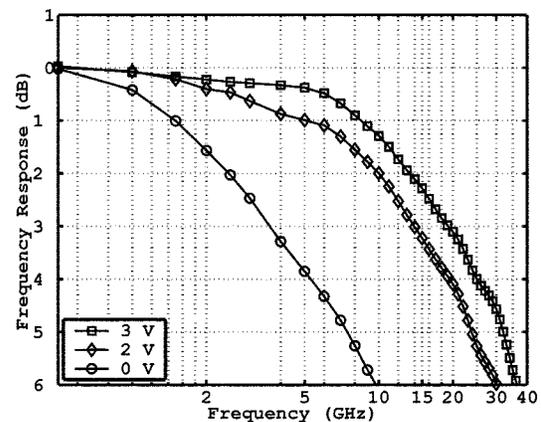
Fig. 4. The FFT of the temporal response measured at 0 V, 2 V, and 3 V dc reverse bias from a 30  $\mu$ m-diameter device. There is a dramatic increase in the bandwidth when the reverse bias is increased from 0 V to 2 V.
