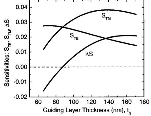
Fig. 2. Waveguide sensitivities versus guiding layer thickness for a silicon nitride–silicon dioxide waveguide ( $n_l = n_u = 1.465$  nm,  $n_g = 2.02$  nm,  $t_l = 1500$  nm,  $t_u = 4$  nm), operating at  $\lambda = 632.8$  nm and a biolayer thickness  $t_b = 10$  nm.
