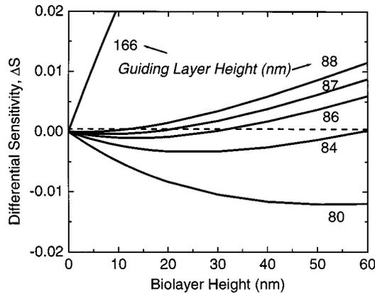
Fig. 4. Waveguide sensitivity versus biolayer thickness, enlarged for thin biolayers for several guiding layer thicknesses. For  $t_g = 87$  nm,  $|\Delta S| < 10^{-4}$  for  $0 < t_b < 25$  nm. Compare to  $\Delta S$  for  $t_g = 166$  nm.
