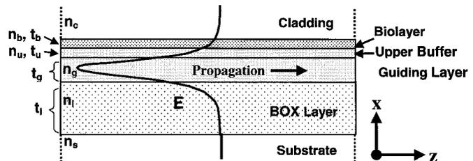
Fig. 1. Generic slab waveguide structure. Thicknesses  $t_x$  and refractive indexes  $n_x$  in each layer vary. BOX is buffered oxide layer and forms first buffer layer. Typical thickness values:  $t_l \simeq 1500 \text{ nm}$ ,  $t_g \simeq 150 \text{ nm}$ ,  $t_u \simeq 5 \text{ nm}$ ,  $t_b \simeq 10 \text{ nm}$ .  $\text{TE}_0$  mode electric field profile displayed. Mode propagates in  $+z$  direction.
