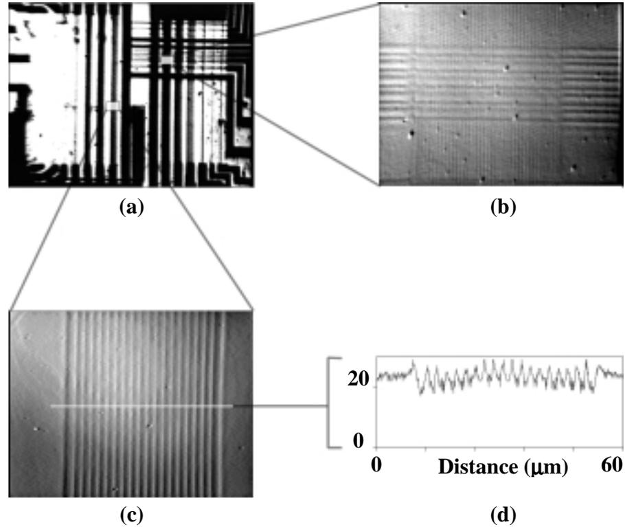
Figure 3. (a) Standard Optical Microscopy (b) NAIL microscopy of vertical poly-silicon lines (c) NAIL microscopy of vertical n-diffusion lines (d) Line cut of data from last image.
