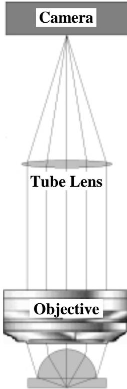
Figure 2. NAIL microscope configuration.
