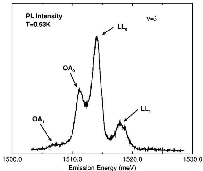
FIG. 2. Individual spectra at  $\nu=3$  displaying low-energy anomalies  $OA_0$  and  $OA_1$ . The fundamental recombinations from the 0th and 1st Landau level are labeled  $LL_0$  and  $LL_1$  respectively. Note the strong intensity of the  $OA_0$  peak relative to the fundamental  $LL_0$ .
