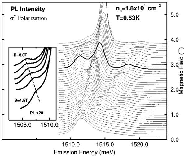
FIG. 1. Photoluminescence spectra in the LCP ( $\sigma^-$ ) polarization at  $T=0.53$  K for the SQW with  $n_s=1.8 \times 10^{11} \text{ cm}^{-2}$  and  $\mu=2.6 \times 10^6 \text{ cm}^2/\text{Vs}$ . The spectra at  $\nu=3$  is highlighted to show the low-energy fine structure. The inset to Fig. 1 displays the lowest-energy feature tuning to lower energy for increasing magnetic field.
