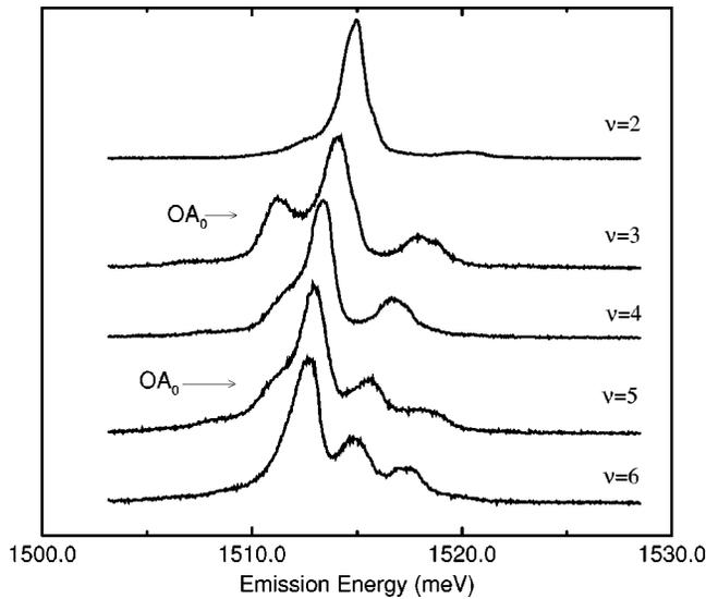
FIG. 4. Magnetic-field development of optical anomalies between  $\nu=6$  and  $\nu=2$ . All spectra are taken in the  $\sigma^-$  polarization at  $T=0.53$  K. For ease of comparison, all spectra have been normalized to have the same peak intensity in the  $LL_0$  transition.
