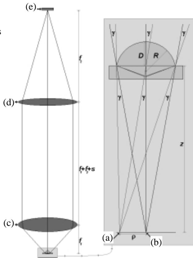
Fig. 7 NAIL microscope configuration.
