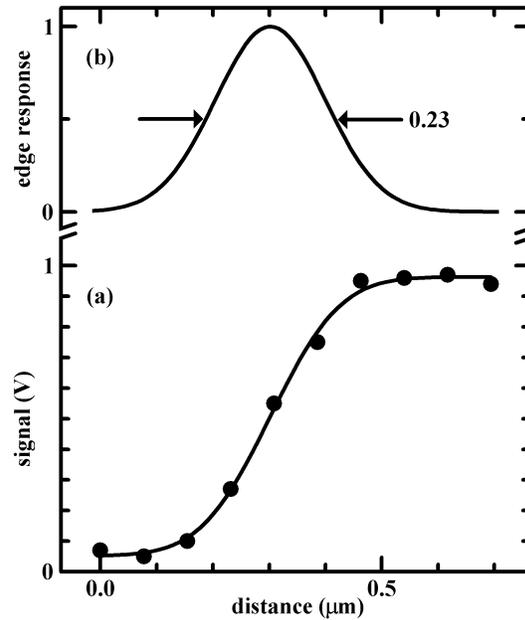
Fig. 11 Horizontal line cut of an edge (a) detector signal plotted by distance in the horizontal direction (b) fitted edge response.
