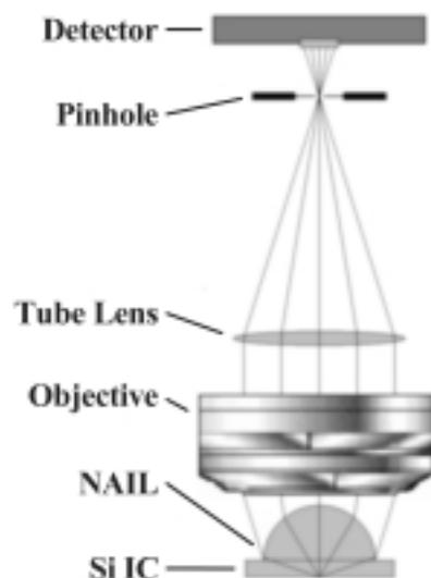
Fig. 9 NAIL microscope.
