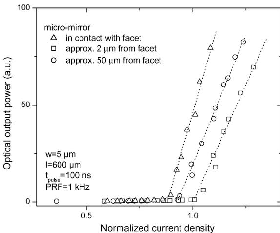
Fig. 4.  $L$ – $I$  characteristics of an uncoated laser in dependence of the micro-mirror position. Output power  $L$  as measured from the uncoated facet. Threshold current reduction and increasing slope efficiency are achieved by increasing the effective reflectance of the opposite facet by means of a micro-mirror.
