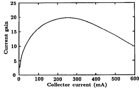
FIG. 2. Dependence of the current gain on the collector current  $I_C$  for HBT<sub>B</sub> with  $V_{CE} = 6$  V and at 300 K.
