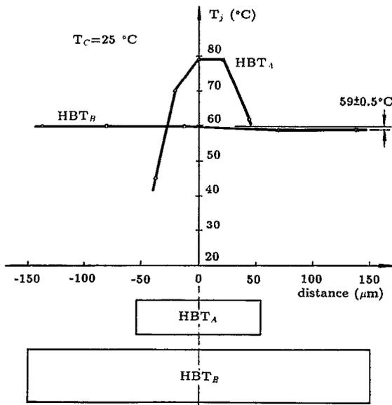
FIG. 3. Surface temperature distribution for HBT<sub>A</sub> at 10 V, 100 mA and HBT<sub>B</sub> at 10 V, 200 mA measured by infrared microradiometer.
