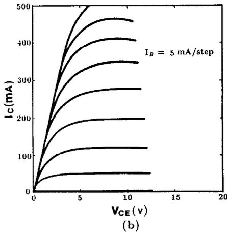
FIG. 1. Typical common-emitter current-voltage characteristics of power HBT<sub>A</sub> (a) and power HBT<sub>B</sub> (b).
